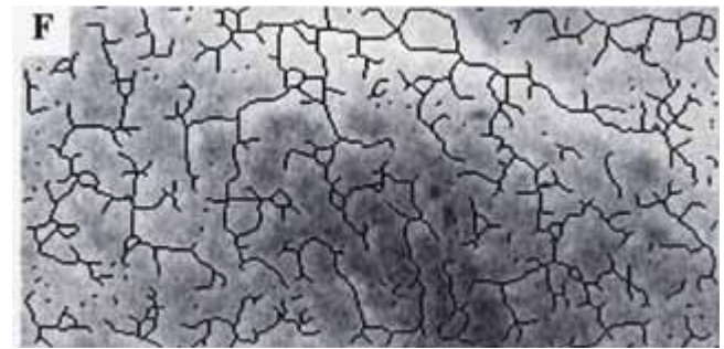
FIGURE 5F. This image shows the skeletonized image in 5e superimposed on the original image (Figure 5a) to show the congruence of the two images.
