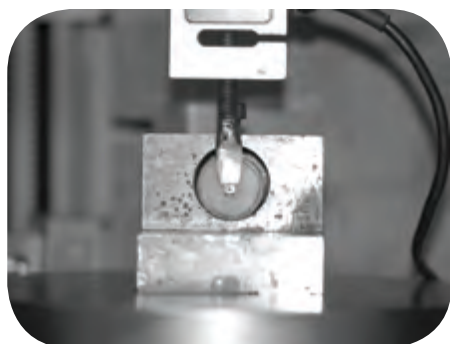
FIGURE 1. A sample mounted on Zwick testing machine and ready for shear testing.
