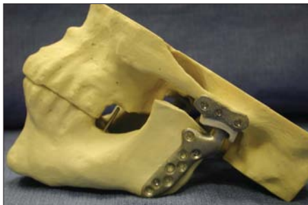
Figure 5. CAD Cam construction model of custom TMJ replacement.
