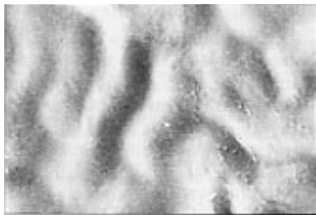
FIGURE 3. Scanning electron micrograph of new tubing prior to placement in the dental unit (8000x magnification).
