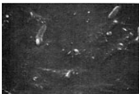
FIGURE 6. Biofilm buildup in the handpiece waterline tubing after six weeks of treatment with Bio 2000 (8000x magnification).
