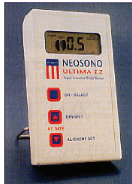
FIGURE 1. Ultima EZ dual-circuitry third-generation apex locator.
