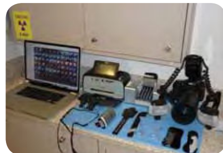
FIGURE 2. A portable digital dental office consists of a digital SLR with macro lens and dual-point flash, photo printer, and a laptop computer with imaging software.
