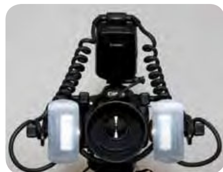
FIGURE 4. A modern dSLR camera equipped with a macro lens, dual-point macro flash, and bracket. This camera (Canon 7D) is also capable of recording HD video when needed.
