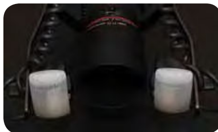
FIGURE 7. A dual-point macro flash system allows each flash head to be positioned further away from the axis of the lens which enhances the fidelity of the image. This is essential in photographing anterior teeth to capture the subtleties of chroma, surface anatomy and translucency. The flash heads can also be moved in close to the lens axis, useful for posterior mirror images.
