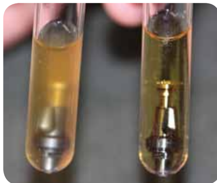
FIGURE 5. Positive and negative controls (impression copings) after incubation at 37 degrees Celsius.
