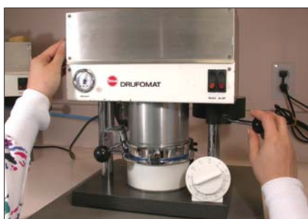
Figure 11. Pressure is used on the first layer and timing is crucial to maintain pressure.
