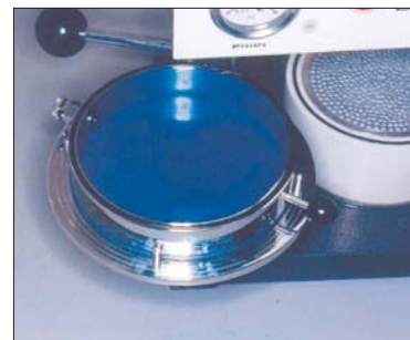
Figure 8. A clamping ring locks sheet into place.
