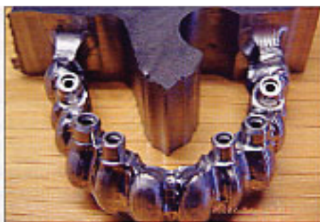
FIGURES 2. Solid milled titanium framework, prior to metal finishing.
