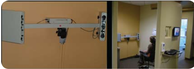
FIGURE 1. This figure shows the active stereophotogrammetry 3dMDface system created by 3dMD (Atlanta, Ga.) and installed using a wall mount strategy at DDI in Roseville, Calif. The system has the option of being portable. The 3dMDface system uses four-machine vision 2 Mpixel sensors for capturing geometry and two-machine vision sensors for capturing texture. The options for the texture sensors are either 2 or 5 Mpixels each. The six sensors simultaneously capture the facial anatomy in 1.5 milliseconds. The capture volume can be up to 0.5 x 0.6 x 0.5 meters. The accuracy has been tested within 0.2 mm depending on the lens configuration. 5
