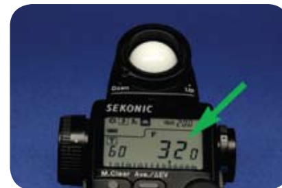
FIGURE 6. An incident light meter can be utilized to measure the intensity of light falling on its sensor. The digital display identifies the proper aperture setting for a perfect exposure with the available light at that working distance, in this case, f32. (See green arrow).
