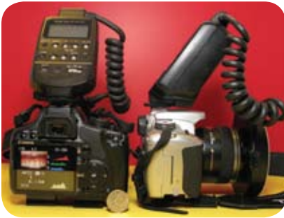
FIGURE 1. Two entry-level Canon SLR clinical camera bodies. The Canon XSi (12 megapixel) on the left and XTi (10 megapixel) on the right. Both cameras are light and have a small profile. Canon ring flash and 60 mm macro lens attached to complete the system as a close-up clinical camera.
