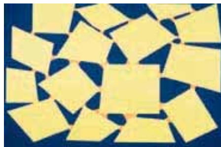
FIGURE 3. During sintering the alumina particles fuse together at points of contact producing a highly stable, organized crystalline structure.
