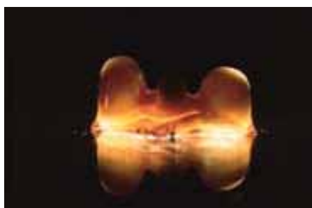
FIGURE 8. Transillumination reveals increased translucency resulting from glass infiltration procedure.
