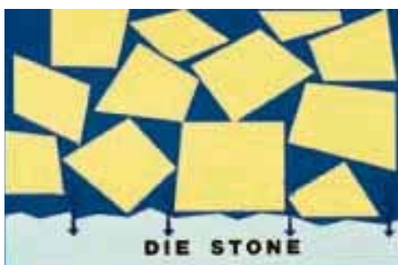
FIGURE 2. Moisture absorbed into die stone agglomerating or packing alumina particles.
