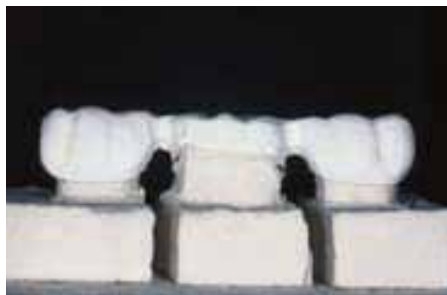
FIGURE 5. Substructure has been sintered. Note how moisture has been driven off and the die has shrunk away from core.
