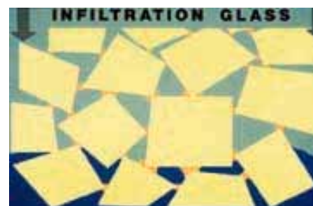
FIGURE 6. At elevated temperatures, infiltration glass moves inside from external surface to fill air spaces between particles by capillary action.
