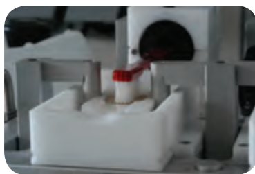
FIGURE 2. Toothbrush with dentin sample mounted in the toothbrush machine.
