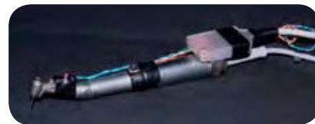
FIGURE 3. Sensor mounted on surgical handpiece.
