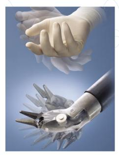
The da Vinci Surgical System's EndoWrist instrument tips can rotate like the human wrist, allowing surgery in the closed chest, abdomen or pelvis.
