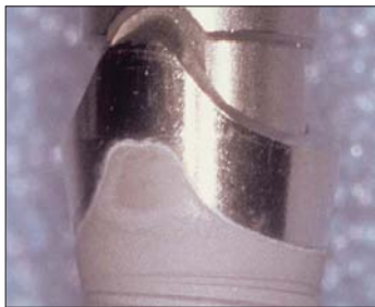
Figure 3b. The platform of the scalloped implant. The platform has a facial level, which is more apical than the interproximal area to follow the anatomic contour of the alveolar bone crest in the anterior area.
