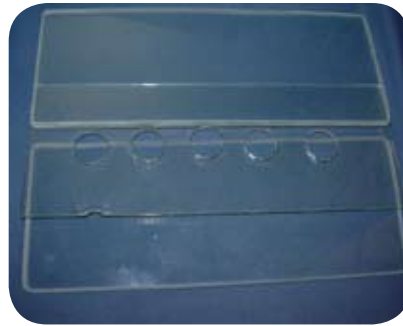
FIGURE 3. A five-hole glass mold was used for the preparation of GC Gradia disks. It consisted of three parts: upper, lower, and a middle hole part.
