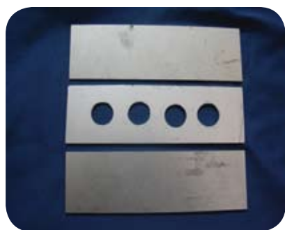
FIGURE 1. A four-hole metal mold was used to prepare porcelain disks.
