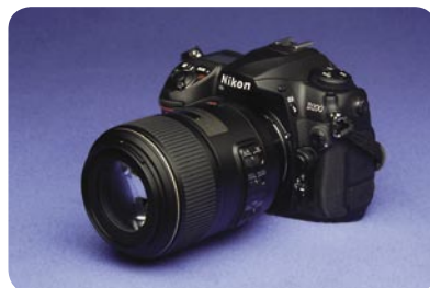
FIGURE 8. Digital single lens reflex camera systems allow use of macro (close-up) lenses with manual focus for repeatable diagnostic magnification. The large camera body can accommodate a large sensor offering high resolution and superior color accuracy.
