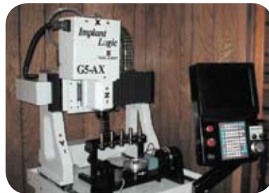
FIGURE 14. Implant Logic computerized milling machine used to manufacture surgical guides. (Image provided by Implant Logic.)
