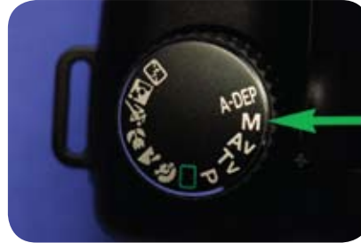
FIGURE 5. The exposure selector wheel of the Canon 30D DSLR is set to manual (M) mode (see green arrow). All other settings represent different TTL (through the lens) exposure strategies that automatically set some (or all) of the camera's exposure controls.
