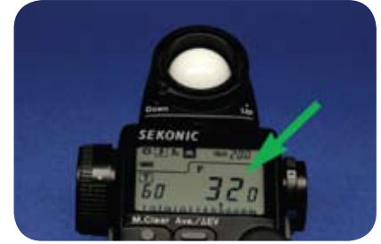
FIGURE 6. An incident light meter can be utilized to measure the intensity of light falling on its sensor. The digital display identifies the proper aperture setting for a perfect exposure with the available light at that working distance, in this case, f32. (See green arrow).
