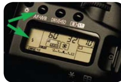
FIGURE 8. The Canon 30D is one of several DSLR cameras that has an external button allowing convenient access for manually selecting the camera's white balance (in this case set to flash, see green arrows).
