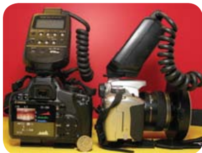
FIGURE 1. Two entry-level Canon SLR clinical camera bodies. The Canon XSi (12 megapixel) on the left and XTi (10 megapixel) on the right. Both cameras are light and have a small profile. Canon ring flash and 60 mm macro lens attached to complete the system as a close-up clinical camera.
