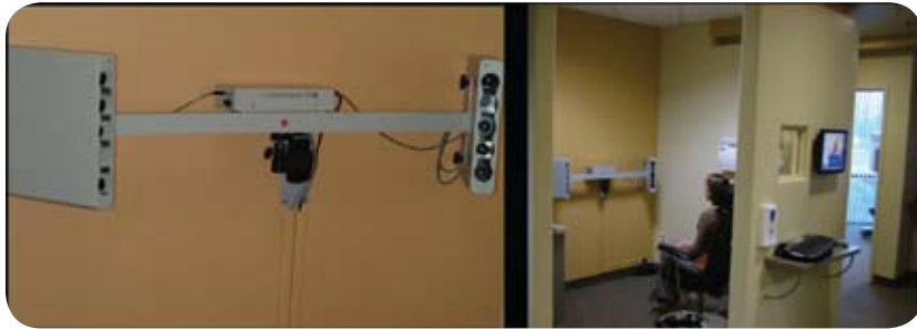
FIGURE 1. This figure shows the active stereophotogrammetry 3dMDface system created by 3dMD (Atlanta, Ga.) and installed using a wall mount strategy at DDI in Roseville, Calif. The system has the option of being portable. The 3dMDface system uses four-machine vision 2 Mpixel sensors for capturing geometry and two-machine vision sensors for capturing texture. The options for the texture sensors are either 2 or 5 Mpixels each. The six sensors simultaneously capture the facial anatomy in 1.5 milliseconds. The capture volume can be up to 0.5 \times 0.6 \times 0.5 meters. The accuracy has been tested within 0.2 mm depending on the lens configuration. 5
