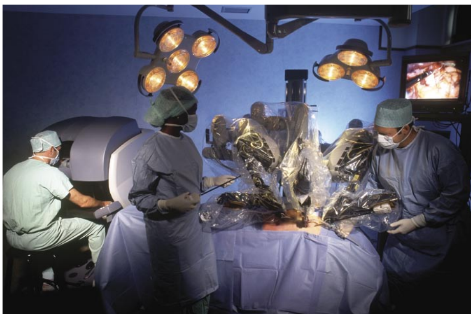
The da Vinci Surgical System is a robotic platform that consists of a surgeon's console, a patient-side cart with four interactive robotic arms, a high-performance vision system and EndoWrist instruments. Photo Copyright 2006 Intuitive Surgical, Inc.
