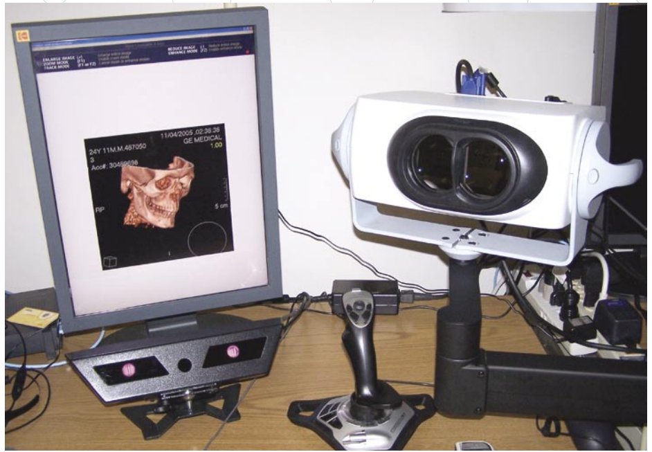
Above is a prototype of the 3-D Stereo Display, which responds to pupil commands of the viewer and does not require goggles. The equipment enables clinicians to feel they are immersed in the image. Photo courtesy of Health Group Technology Innovation, Eastman Kodak, Rochester,
