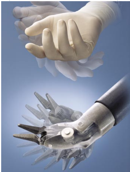
The da Vinci Surgical System's EndoWrist instrument tips can rotate like the human wrist, allowing surgery in the closed chest, abdomen or pelvis.
