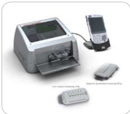
FIGURE 8. The UCLA oral fluid nanosensor test (OFNASET): Showing two chips, one for oral cancer screening and one for Sjögren syndrome screening (courtesy of Dr. David Wong).
